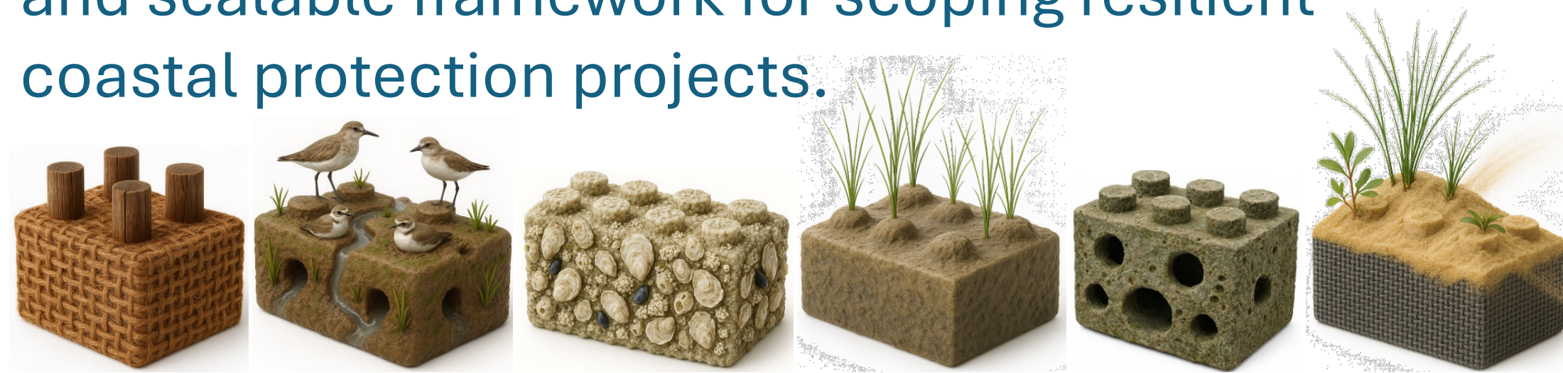
Figure 1. Typical nature-based solutions (from left to right): coir edging, marsh restoration with hydrologic connectivity, living breakwaters, dredge material beneficial use, oyster reefs, and beach and dune nourishment
